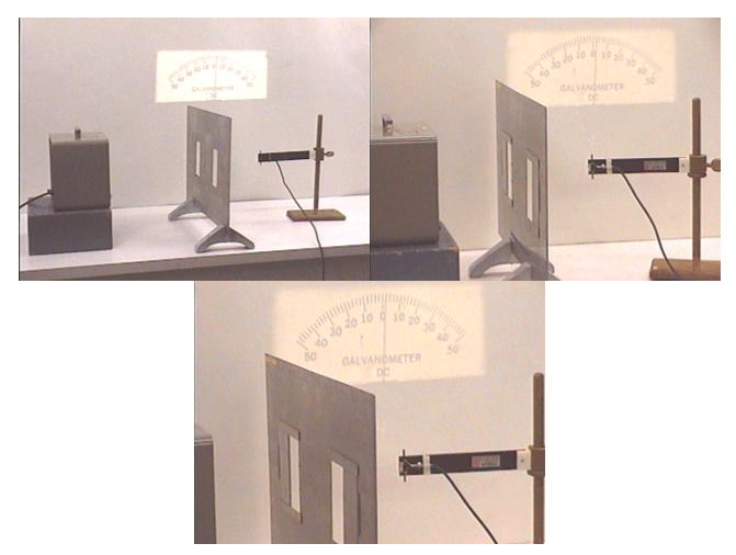
The distance from the source to both of the slits is equal. The distance from the front slit to the detector antenna, seen in the photograph at the left below, is about 26 cm, while the distance from the rear slit to the receiver is about 20 cm, as seen in the photograph at the right. The wavelength of the microwave source is about 12 cm. There seems to be about one microampere of microwave radiation coming through the two slits to the antenna, as seen on the microammeter in the pictures above.
